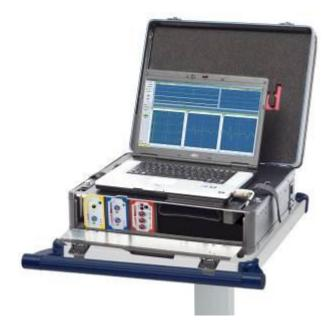
The ISIS IOM portable consists of a suitcase, a laptop, the new ISIS Neurostimulator and ISIS Headboxes. This configuration is especially suitable for portable applications or where space in the OR is limited.
